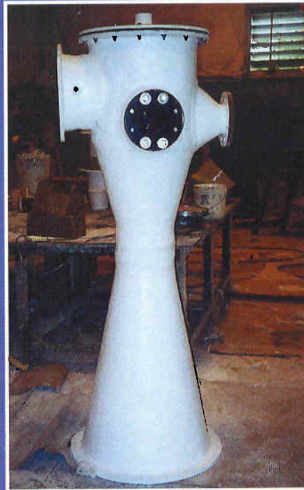
Emergency Chlorine Venturi Scrubber
